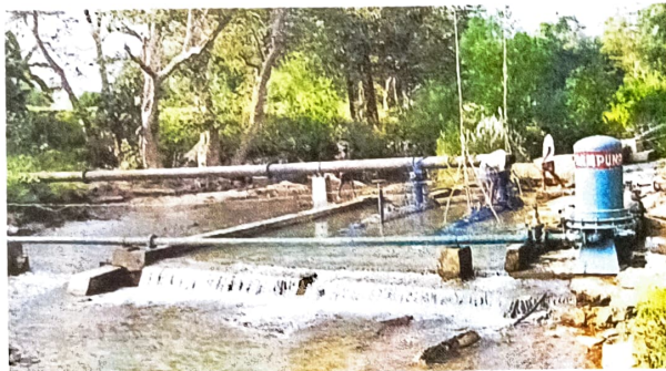
The turbine uses about 90% of the river water flow at low head, which is then recycled back to the river, to generate power.
